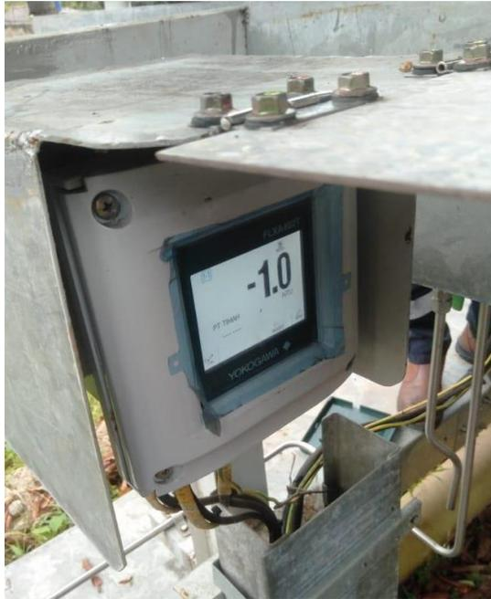
*Gambar 2. 6 Hasil Monitoring Nilai Sensor Turbiditi*
