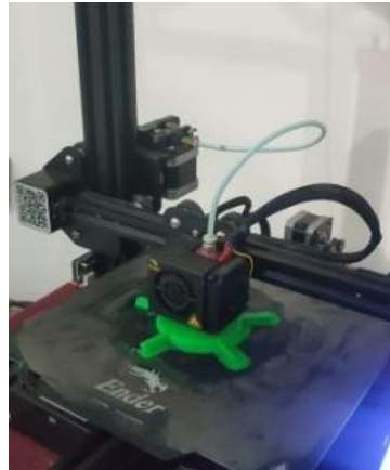
Gambar 3. 9 Proses Percetakan Prototype Waterjet Thruster
