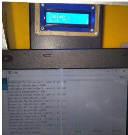
Gambar 4.14 Hasil Pengujian LCD 16 x 2 I2C
