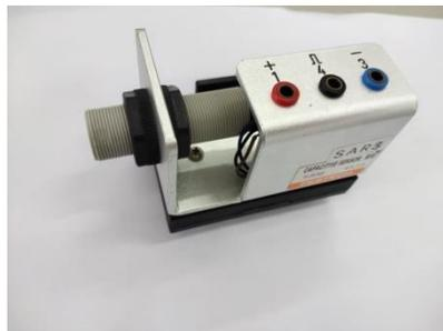
Gambar 2.4 Sensor *Proximity* Kapasitif
