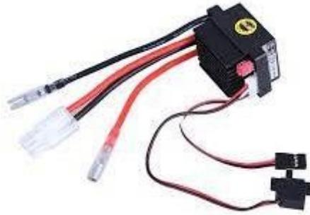
*Gambar 2. 4 Elektonic Speed Control*
