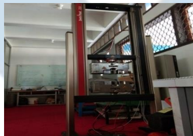
Gambar 3. 10 Mesin Universal Testing Machining merek Zwick Roell Z020 tipe Xforce K
