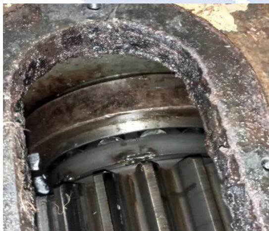
Gambar 2.7 Bearing Gearbox Spull Gear Mesin Screw Press (Sumber: PT Gunung Maras Lestari, 2023)
