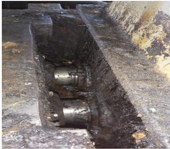
Gambar 2.6 Oil Seal Gearbox Reduser Mesin Screw Press (Sumber: PT Gunung Maras Lestari, 2023)
