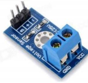
Gambar 2. 3 Sensor Tegangan[3]
