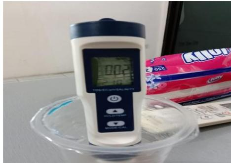
Gambar 3. 4 Alat Salinitas Tester
