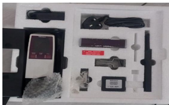
Gambar 3.5. Surface Roughness Tester type Mitutoyo SJ-210
