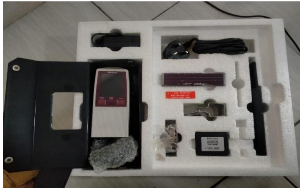
Gambar 3. 6 Surface Roughnes Tester
