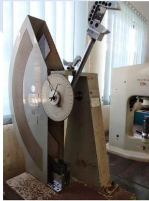
*Gambar 3. 4Alat Uji Impak*
