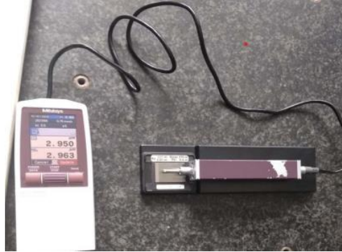
Gambar 3. 15 Proses Kalibrasi Surface Roughness Tester
