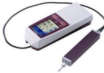
Gambar 3. 4. Surface roughness tester SJ-210
