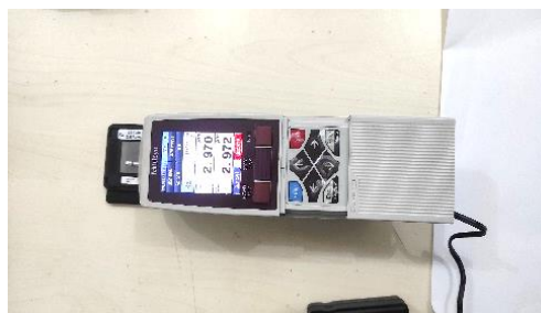
Gambar 4. 10. Kalibrasi surface roughness tester
