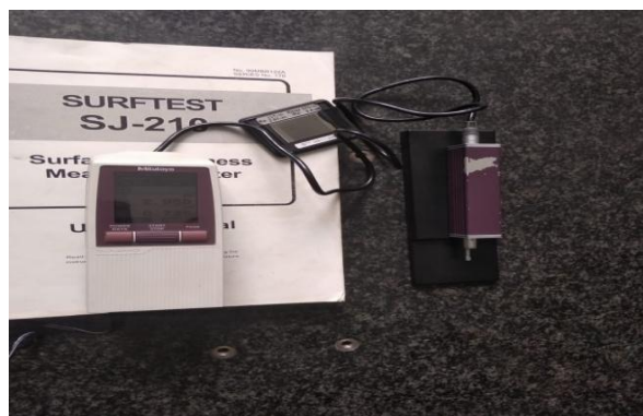
Gambar 3. 2 Surface roughness tester Mitutoyo SJ-210
