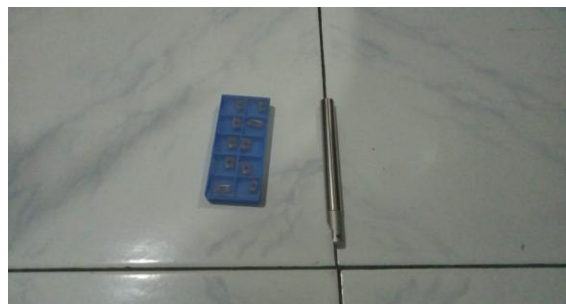
Gambar 3. 6 Insert Carbide Milling APMT 1135
