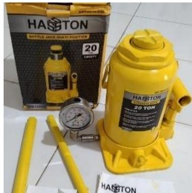
Gambar 2. 1 Dongkrak 10 Ton Dengan *Pressure Guage* HASTON
