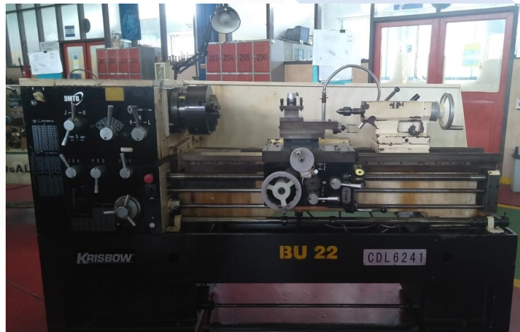
Gambar 2. 2 Mesin Bubut Krisbow Tipe AOB2 – 25 Model CDL6241
