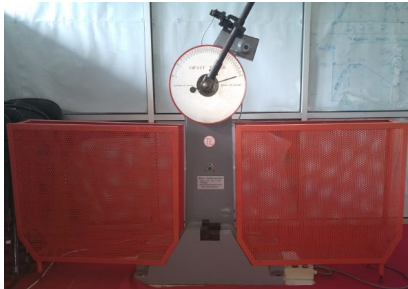
Gambar 4. 7 Mesin Uji Impak Metode Charpy Model JB-300B
