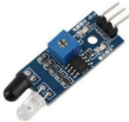
Gambar 2.6 Sensor *Infrared*
