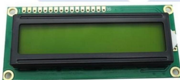
Gambar 2.7 LCD 16x2
