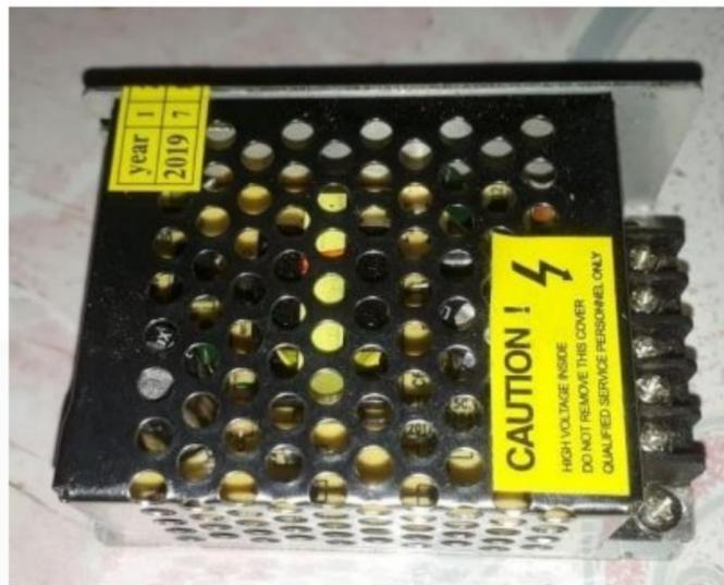
Gambar 2.10 *Switch – Mode Power Supply* 12V
