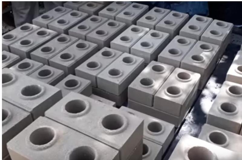
**Gambar 2.1.** *Soil-Cement interlocking block* (*Chundakus Habsya dkk, 2010*).
