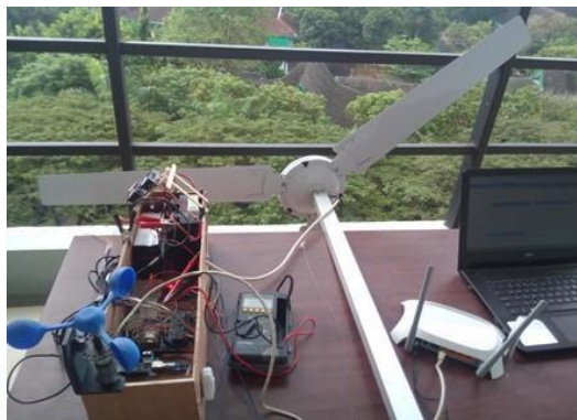
Gambar 2. 2 Sistem Off- Grid Pembangkit Listrik Tenaga Angin berbasis IoT (Internet of Things) [3]
