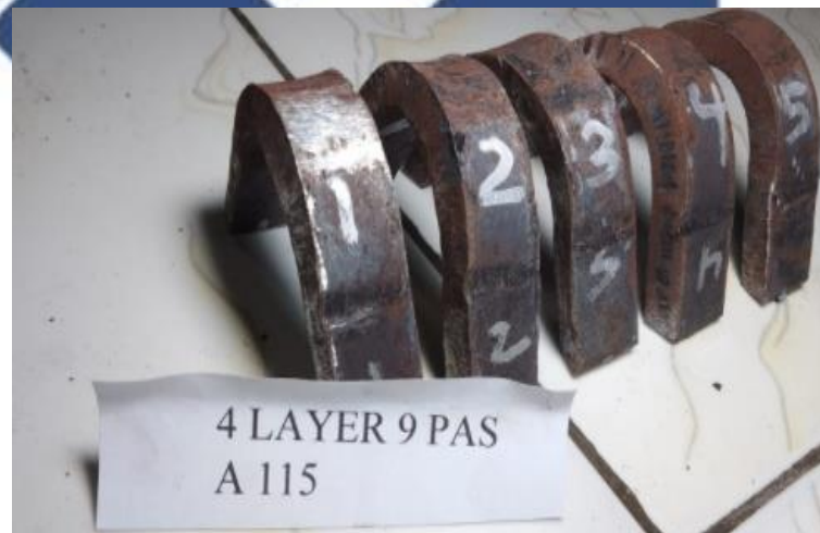
Gambar 4.3.4.3. Hasil Uji Bending 4 Layer 9 Pass 115A
