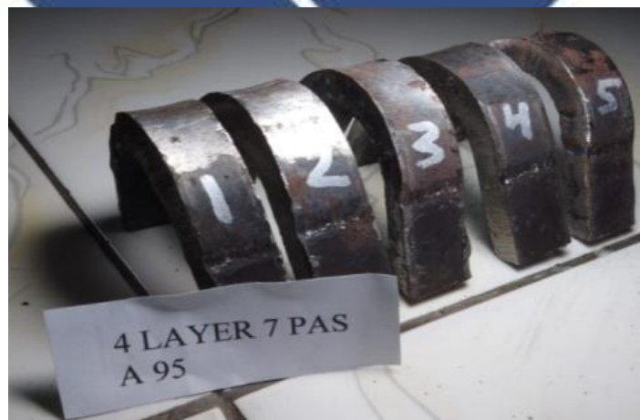
Gambar 4.3.4. Hasil Uji Bending 4 Layer 7 Pass 95A
