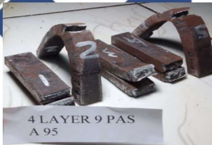
Gambar 4.3.4.1. Hasil Uji Bending 4 Layer 9 Pass 95A
