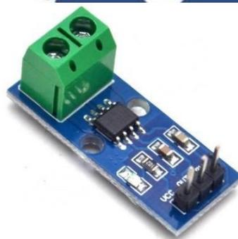
**Gambar 2. 16** Modul Sensor Arus ACS712-30A
