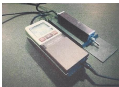
Gambar 3.5 Surface Roughness Tester Type SJ201
