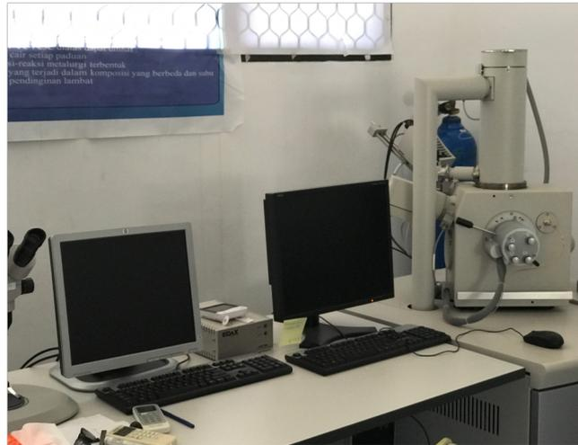
Gambar 2.1 Mesin Uji Sem
