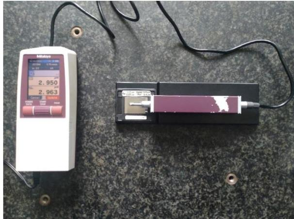
**Gambar 3.3** Mesin *Surface Roughness*
