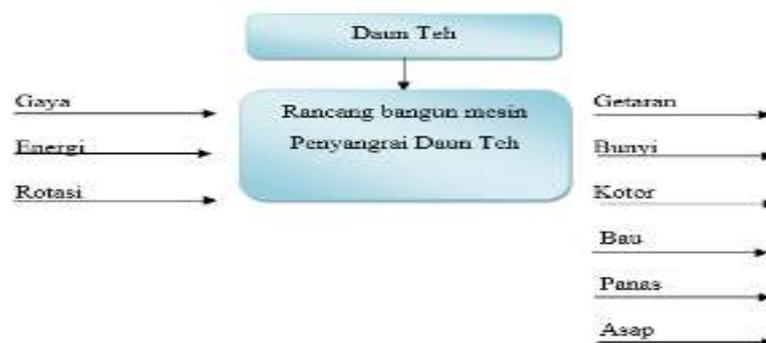
Gambar 4.1 Diagram *black box*/diagram fungsi
