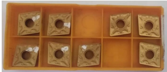
Gambar 3.5 Pahat Insert Carbide CNMG 120408-MA
