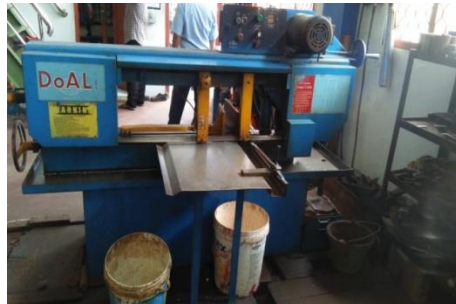
Gambar 3.2 Mesin Gergaji Potong DOALL Model C-916
