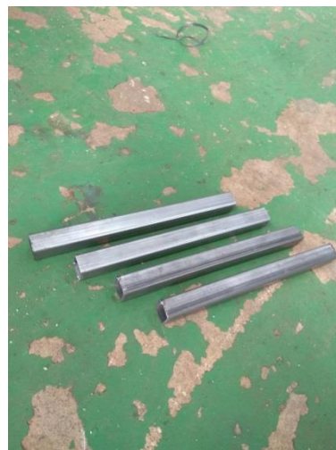
Gambar 4.1 Material Baja St37 Hollow
