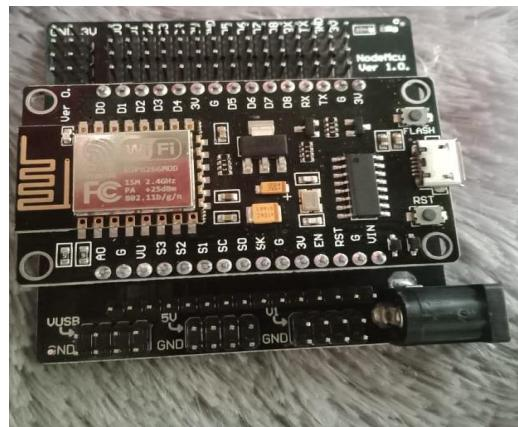
Gambar 2.5 NodeMCU ESP8266
