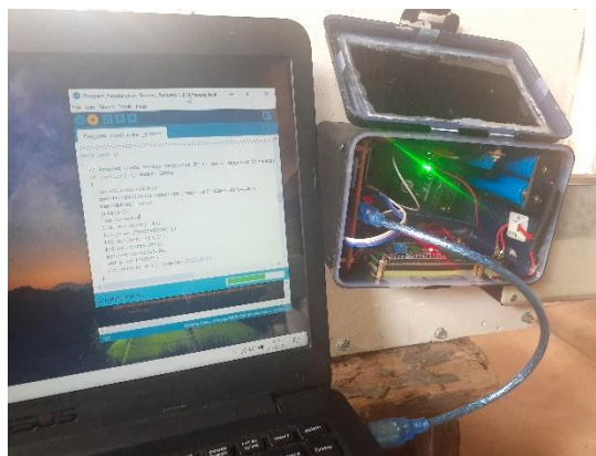
Gambar 4.14 Proses upload program menggunakan kabel downloader
