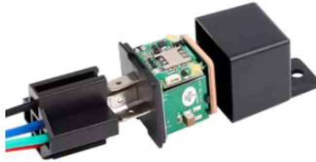
Gambar 2.6 CJ720 Versi Global Relay GPS Tracker [10].
