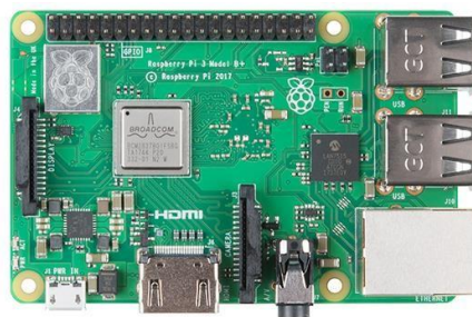
Gambar 2. 6 Raspberry pi 3 B+ [12]
