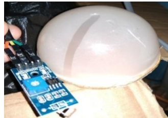
Gambar 4.22 Modul sensor LDR
