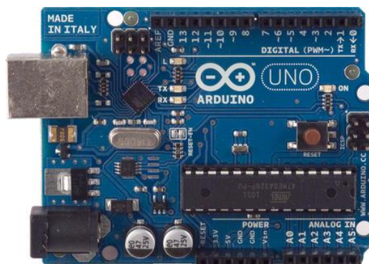
Gambar 4.5 Board Arduino Uno
