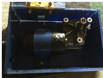
Gambar 4.7 Motor wiper 12V 5A
