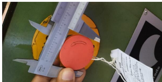
Gambar 4.1 Tombol emergency rusak
