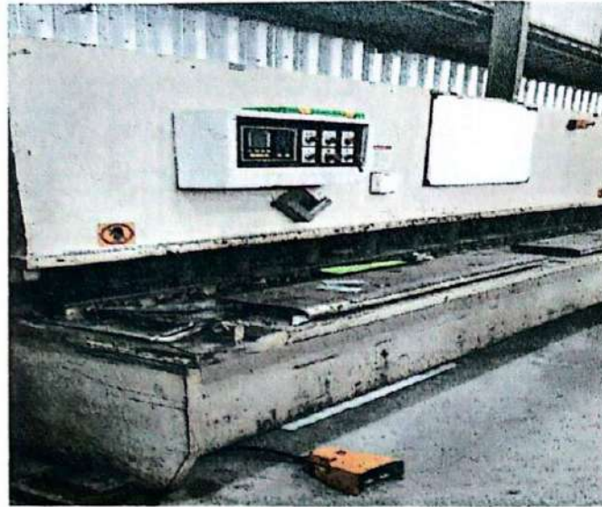
Gambar 1.5 Mesin Shearing Plat
