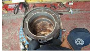
Gambar 2. 8 Pengukuran Outside Diameter Bearing
