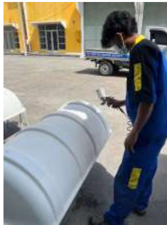
Gambar 2.6 proses Painting cangkang liferaft /kapsul
