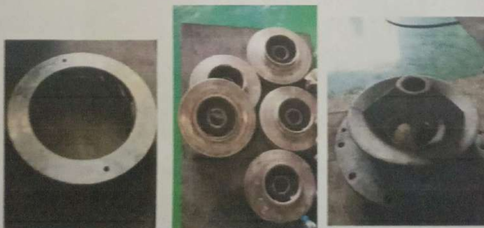
Gambar 16 2.8 Disfusser Casing, Impaller, dan Suction Belt Disfusser
