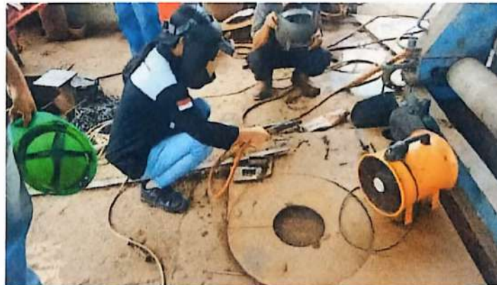
Gambar 2.2 Pengelasan Stainless Screw Auger Rebusan
