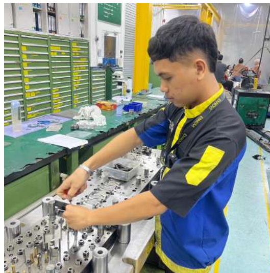
Gambar 2.2 proses pengecekan Punch
