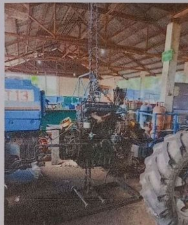
Gambar 2. 4 Overhaul traktor landini 8860
