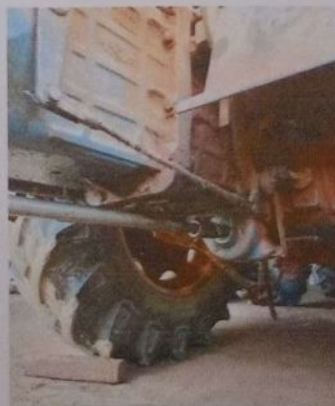
Gambar 2. 6 Ganti seal as Panjang gardan traktor landini 8860
