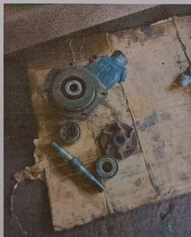
Gambar 2. 17 perbaiki water pump traktor landini 8860
