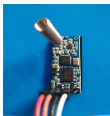
Gambar 4.32 *Radio Frequency HC-12*
