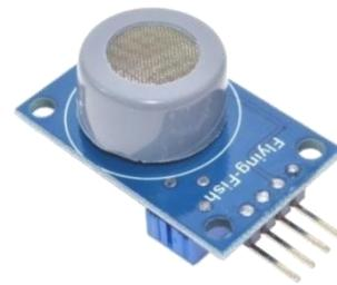
Gambar 2.4 Sensor MQ7 (*Pixel Electric Engineering, 2018*)
