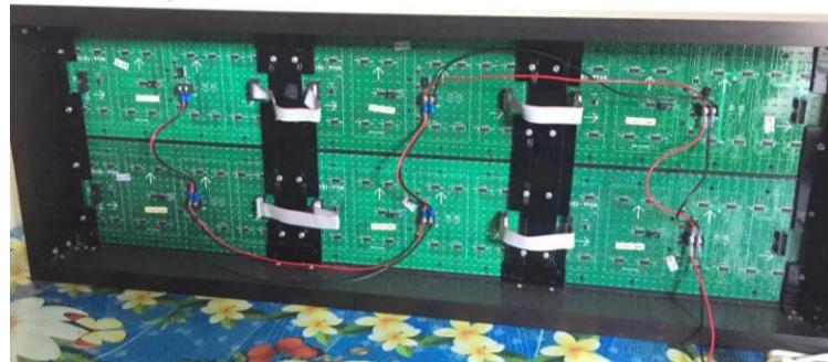
Gambar 4.4 *Frame DOT Matrix Display* Tampak Belakang
