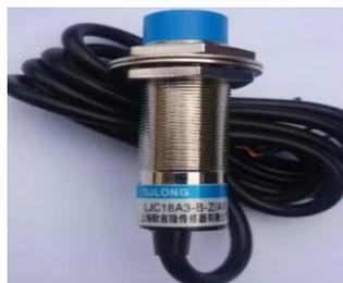
Gambar 2.9 Sensor *Proximity Kapasitif* (OFstore, 2025)
