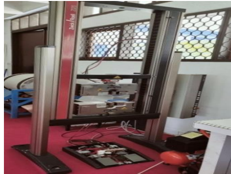
Gambar 3.5 Mesin Uji Tarik ( Zwick Roell )
