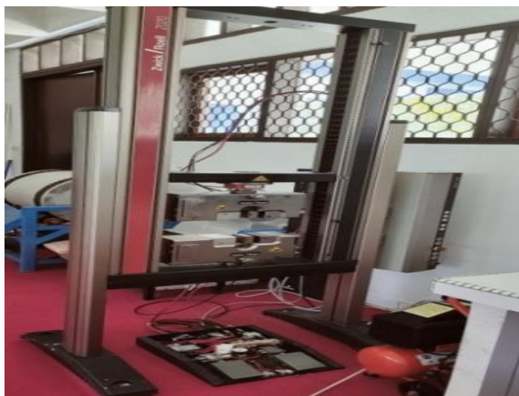
Gambar 4.1 Mesin Uji Tarik ( Zwick Roell )
