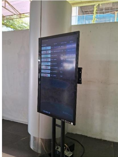
Gambar 2.8 Flight Information Display System (FIDS)
