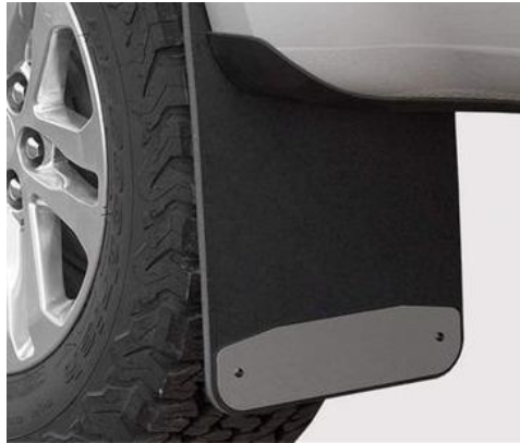
Gambar 2.16 Spakbor Skirt Mobil (Sumber: www.gridoto.com )
