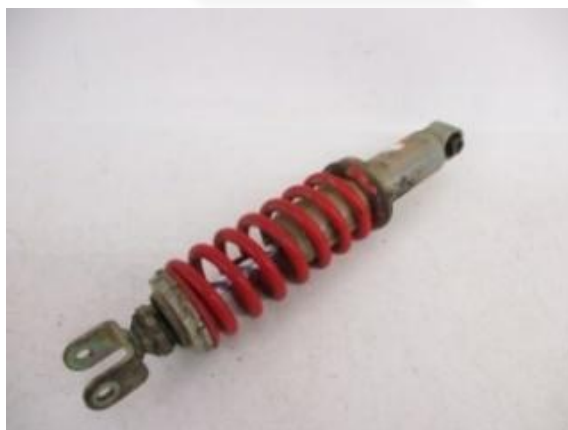
Gambar 2.17 Shock Absorber (Sumber: https://www.cyclesrus.net )
