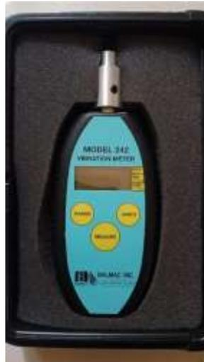
**Gambar 4.2** *Vibrometer*
