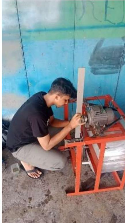
**Gambar 4.9** *Alignment Pulley*
