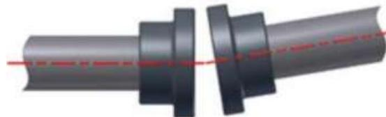
**Gambar 2 2** *Missalignment angular*/menyudut
