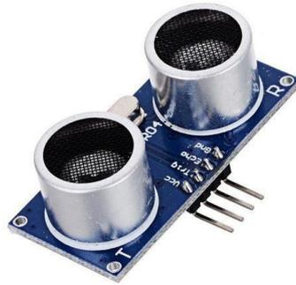
Gambar 2.7 Sensor Ultrasonik
