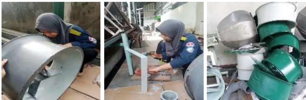
*Gambar 2. 4 Proses pengecatan/*painting**
